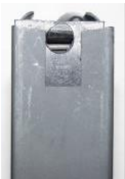
Gen I magazine with spring loaded bolt catch trip
